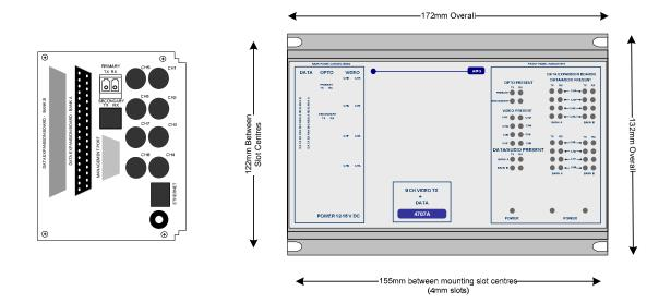
The **AMG4707A** is a rackmount data transmit unit designed to transmit and receive up to 8 data or audio signals over two singlemode fibres. The 8 data/audio channel interfaces, whether RS232, RS422, RS485, 20mA, TTL, Contact Closure, Lonworks or Audio, are defined at manufacture by the addition of daughter boards fitted onto the Data Expansion Board A.
